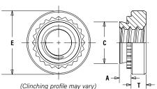
Due to manufacturing procedure, parts may have a counterbore at shank end.
