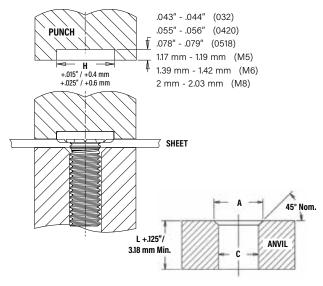
Tooling for sheet thicknesses .060" / 1.51 mm and greater with #10 / M5 and 1/4" / M6 thread sizes and .075" / 1.9 mm and greater with 5/16" / M8 threads.
