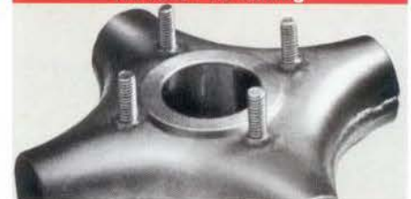
Homogeneous full fusion weld
