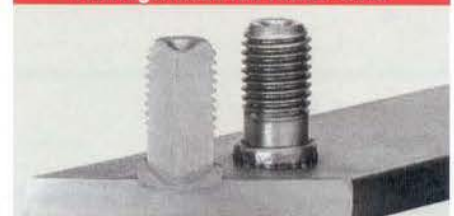
Homogeneous full fusion weld
