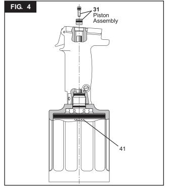
locking Nut (41) with 9/16 socket and extension and torque Screw (32) using 7/64 hex key to 55-60 in. lbs. Torque Nut (41) to 28-32 ft. lbs.
